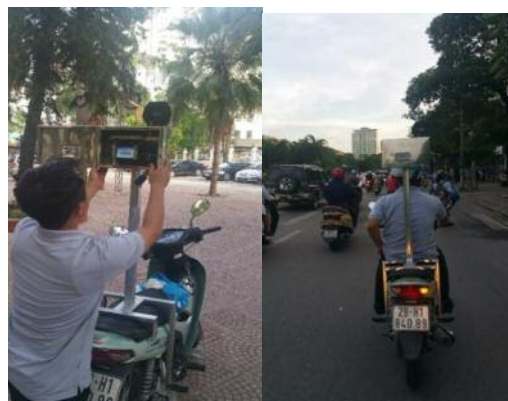
Fig. 11. Mobile dust monitoring by motorcycles
