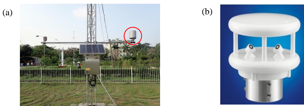
Figure 5. (a) An appearance of WB AWS system (Vinh Regional Hydro–Met Center). The rain gauge sensor is shown in red circle. And (b) wind speed and direction sensor settled at the top of the 10m tower.
