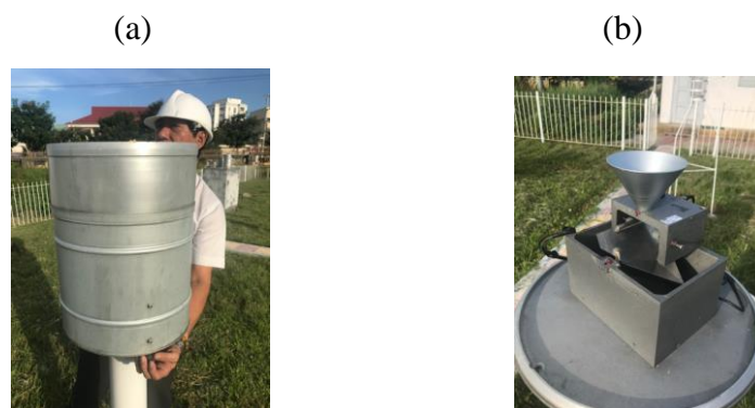
Figure 9. (a) Appearance and (b) inside view of rain gauge (PMB2) of Italian AWS (Da Nang Regional Hydro–Met Center).
